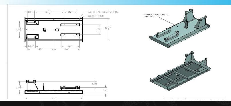
Axis Mechanical Group can design and fabricate pump bases for our customers desired specs and measurements.
